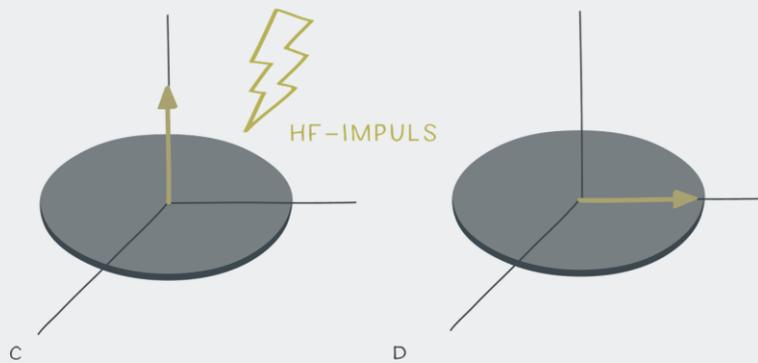
**Figure 3:** Spin and magnetic moment of a proton\*
